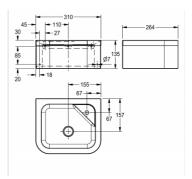
Drinking water fountains are manufactured from grade austenitic stainless steel, material thickness 1.2mm, supplied complete with 19mm waste and water bubbler. The wall mounted model is simply fixed to the wall using a joggle strip and integral mounting brackets.
