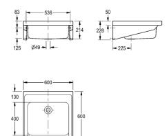
A single bowl sink manufactured from 1.2 mm thick, grade 1.4301 (304) stainless steel, satin polish finish. The sink top is turned down on all four edges and incorporates a wet area recess. The bowl is prepared for a 38 mm waste outlet.
